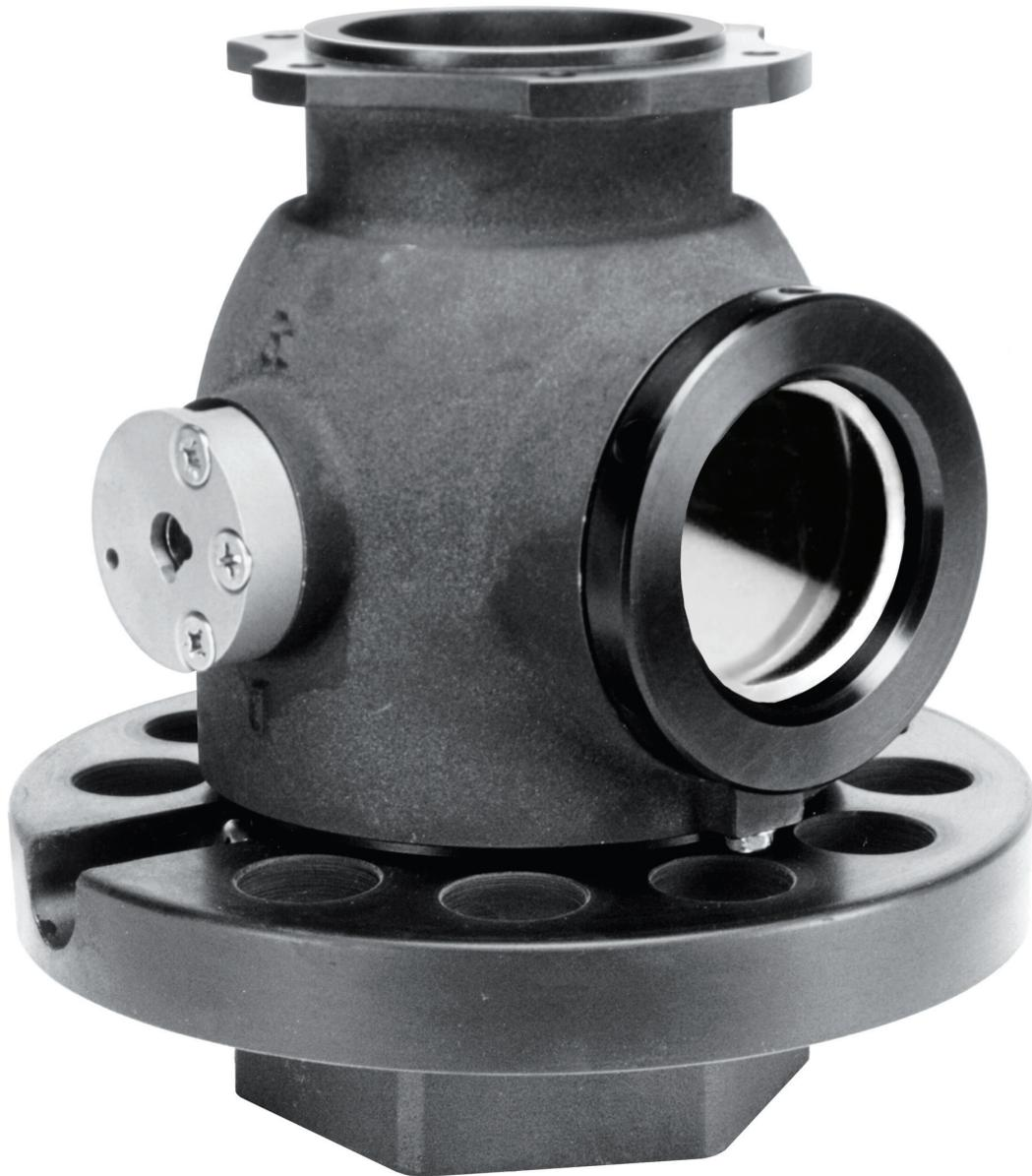
Eaton's Carter Model 64015 Ball Valve is designed to mate with various manufacturers' underwing refueling nozzles to provide ease of strainer inspection and to add a true swivel action to the combination unit. Model 64015 is available with a variety of options for customizing the unit to fit various requirements. In one form, the strainer can be checked without the spillage of any fuel. In its simplest form, fuel spillage caused by the checking of the strainer is minimal.
